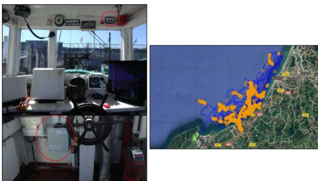
Figure 5 : Energy and vessel monitoring device onboard the Itsas Belhara
