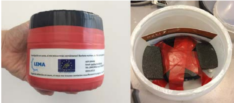
Figure 16. External appearance and internal assembly of low-cost drifting buoys
